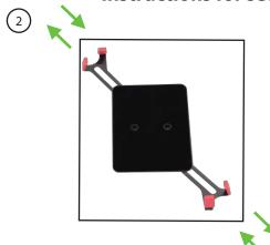
The Tab Grabber has grabber arms at the bottom left and the top right that extend in and out to accomodate different tablet sizes.
