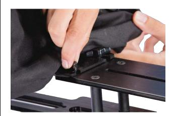
Slide the hood/glass assembly onto the front of the teleprompter sled. The slotted tongue will slide under the 2 thumb screws. Once the hood is in place tighten the 2 thumb screws down to secure hood/glass assembly
