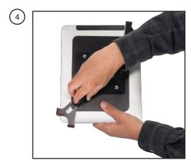
While pushing in both extension arms to keep the iPad in place turn over. Tighten both thumbscrews to keep extension arms in place.
