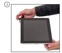
Place the tablet in the Tab Grabber. Press the extension arms firmly against the tablet to give a snug fit.
