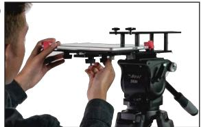
Slide the Tab Grabber to the desired position and tighten the two thumbscrews to secure in place.
