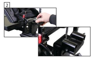
Attach 15mm Rail Mount Adapter using a flat head screwdriver, and the flush screw.
