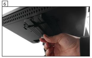
Securely lock the Monitor onto the Front Sled and Reset your Catch Screw to ensure the Monitor will safely remain secure.
