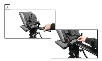
Attach the Back Sled and Screw it into place. The thumbscrew requires no tools. If you have a smaller camera / lens setup and need to get it closer to the beampslitter glass use the flush screw, which will require a Flat Head screwdriver or a Quarter.
