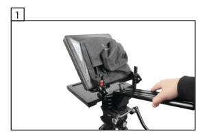
Remove the Backsled, and take the Teleprompter off of the tripod. You can Remove the Monitor and Glass for safety, if you leave it on ensure you are taking care to protect the monitor and beamsplitter glass.
