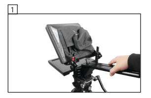
Remove the Backsled, you can leave the Teleprompter on the Tripod.
