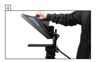
Pull hood, to a 45° Angle. This Angle should allow you to set your red tabs down into their their slots. This will lock the Hood in at a 45° Angle. Then tighten both sets of Knobs on each side. Ensure your Beamsplitter Glass / Hood is properly set before letting it go or allowing it to support it self.
