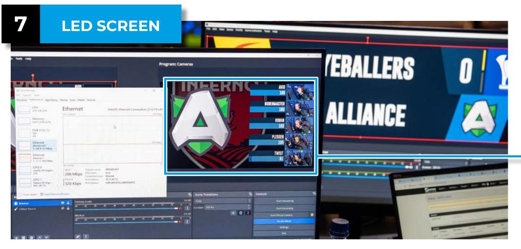
The management of the LED screen was handled by an external team. They employed a dual-computer setup, each running OBS to generate NDI signals for each half of the expansive 40:9 screen. Each feed incorporated five cameras, along with player names and additional data. These NDI feeds were then processed through a computer running Resolume Arena, which was responsible for outputting the final composite image onto the LED screens.
