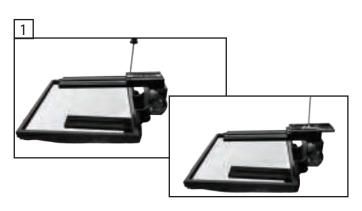
Position our Tripod Adapter Plate and attach your Tripod plate to our Adapter Plate. For smaller cameras under 5lbs attach your Tripod Adapter Plate to the front sled. For larger cameras attach your Tripod Adapter Plate to the back sled. (See Large Camera Setup Tutorial on PrompterPeople's YouTube)
