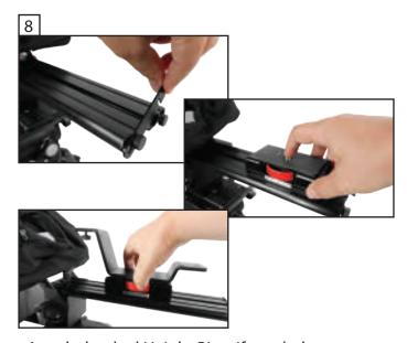
Attach the dual Height Riser if needed, using the included thumb screw. If you need to adjust the position of the dual height riser ensure you are securing your camera with your second hand until your dual height riser is securely set into place.
