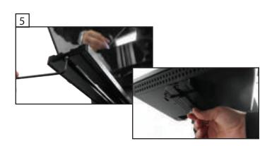
To add your Optional 12" Regular or HighBright Monitor you first need to detach the Catch Screw using a 7/64" Allen Key. Then slide your Monitor onto the front Sled. Securely Reset your Catch Screw to ensure the Monitor will safely remain secure.
