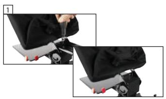
Remove your Camera from the Dual Height Riser Remove the back sled, and take the Teleprompter off of the tripod.
