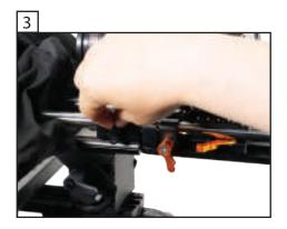
Attach your 15mm Railmount Camera Rig. Lock your 15mm Rails into place on the PrompterPeople 15mm Rail Block.
