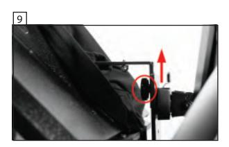
To bring your camera sled up or down to position your camera lens centered to the beamsplitter glass you will need to unscrew the set thumbscrew that is circled in red, and move the camera sled up or down as needed and reset (Screw-in) the thumbscrew to set your sled height.
