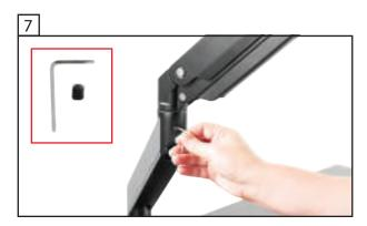
Use the small black locking screw, and the small allen wrench with the flat head screw driver, or use your own flat screw driver to lock the holding screw into place. Do not over tighten it, but tighten it securely so that the top arm cannot be separated from the bottom arm
