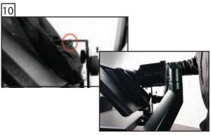
Attach your camera using the thumb screw (Circled in red) to the sled.
