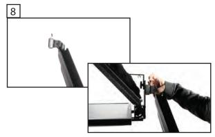
Attach the Teleprompter to the Top Arm by holding back on the locking tab. Slide the Teleprompter fully down and release the tab, this will lock the Teleprompter into place.
