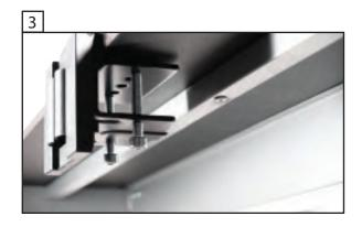
Base properly attached to the back of desktop. Save the Allen Key (Wrench) for adjusting the angle and for any adjustments to the position on your desktop.
